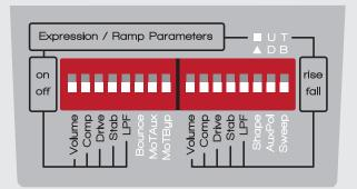
A very important thing to remember is that ramping always gets reset when bypassing. The parameters' current knob position control where the parameters ultimately will either start or stop ramping. **The VOLUME, DRIVE, STAB, COMP, and LPF** dip switches on the left side simply turn that parameter on or off for ramping or expression / CV capability.
