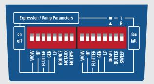
A very important thing to remember is that ramping always gets reset when bypassing. The parameters' current knob position control where the parameters ultimately will either start or stop ramping. **The Wow, HP, Flutter, Gen, and LP** dip switches on the left side simply turn that parameter on or off for ramping or expression / CV capability.
