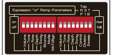
A very important thing to remember is that ramping always gets reset when bypassing. The parameters' current knob position control where the parameters ultimately will either start or stop ramping.
